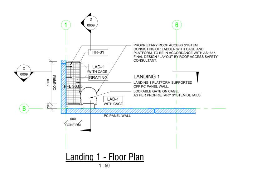
ROOF ACCESS NOTES: 1. PROPRIETARY ROOF ACCESS SYSTEM CONSISTING OF: LADDER WITH CAGE AND PLATFORM, TO BE DESIGNED AND INSTALLED IN ACCORDANCE WITH AS1657. FINAL DESIGN / LAYOUT BY ROOF ACCESS SAFETY CONSULTANT.
